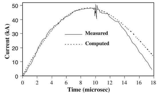
**Fig. 1** Measured (solid line) vs. computed (dotted line) current traces PF-SY1 at 15 kV and 0.38 Torr  $N_2$
