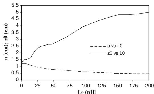
**Fig. 5** Effect on the anode length and inner radius (computed) as  $L_0$  is reduced
