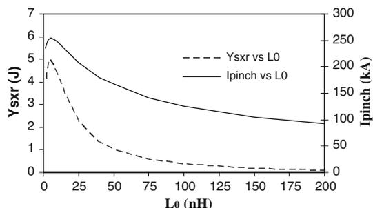
**Fig. 4** The X-ray yield and  $I_{pinch}$  (computed) vs.  $L_0$  (200–1 nH)
