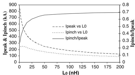
**Fig. 3** Effect of  $L_0$  reduction on currents and current ratio (computed) PF-SY1 at 15 kV, 10 Torr of  $N_2$
