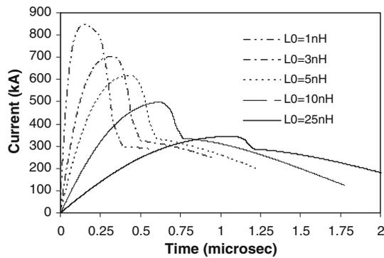
**Fig. 2** Current traces (computed) PF-SY1 at 15 kV, 10 Torr of N<sub>2</sub> for a range of L<sub>0</sub> (25–1 nH)
