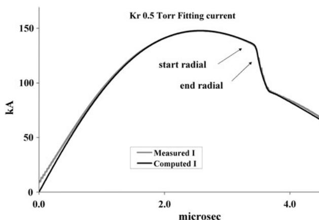
**Fig. 2** Current trace (measured) for krypton at 12 kV 0.5 Torr INTI PF used to fit computed current trace. The good fit is obtained with fitted parameters:  $f_m = 0.035$ ,  $f_c = 0.7$ ,  $f_{mr} = 0.09$   $f_{cr} = 0.7$
