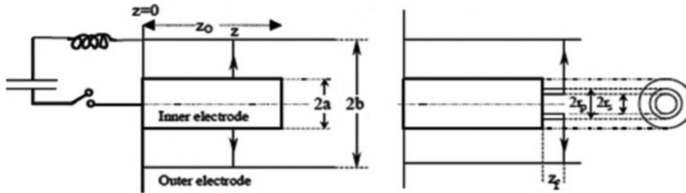
**Fig. 1** Schematic of the axial and radial phases. The left section depicts the axial phase, the right section the radial phase. In the left section,  $z$  is the effective position of the current sheath-shock front structure. In the right section  $r_s$  is the position of the inward moving
