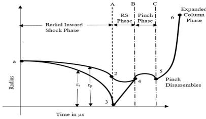
Fig. 2. Radial dynamics. Vertical line A: start of the RS phase. Vertical line B: end RS phase/beginning of pinch. Vertical line C: pinch phase ends.
