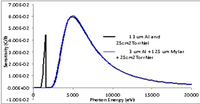
Fig. 4. Two Ch1 and Ch2 channels have the identical sensitivity curves for the spectral range from 1550 eV to 20 keV and beyond. Ch1 has an additional feature sensitivity spike from 900 to 1550 eV not shared with Ch2.
