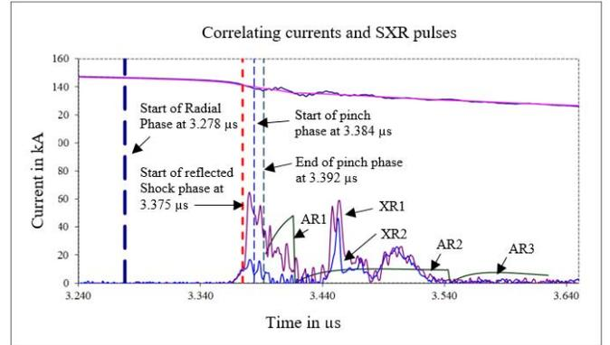
Fig. 5. Correlating the measured characteristic He-like and H-like Ne SXR pulses with the PF dynamics of S14.
