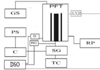
Fig. 3. Block diagram of INTI PF. PFT = PF assembly, GS denotes the supply of gas, PS is the power supply, C is the capacitor, SG is the spark gap, TC is the triggering unit, RP is the rotary pump, D is the voltage divider, RC is the  $dI/dt$  coil, and SXR denotes the DXS spectrometer [19].
