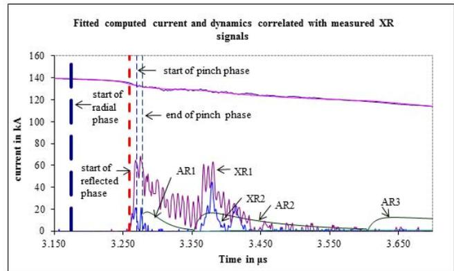
Fig. 1. Correlating the measured Ne SXR pulse (difference pulse of XR1 – XR2) with the fitted computed and measured current traces. The fitting is good and the current traces overlap (top trace).
