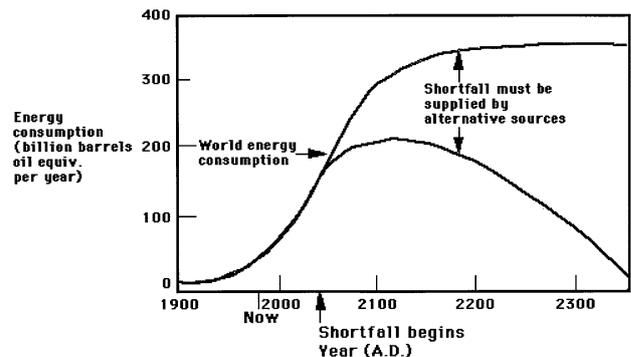
**Fig. 4** Energy consumption versus energy supply based on a stabilized population of 10 billion with average energy consumption per head taken as  $\frac{3}{4}$  of 1985 US per head consumption. The energy supply curve matches the demand curve until just before 2050 when the supply curve becomes unable to meet the demand curve. The increasing shortfall is indicated by the widening gap between the demand (upper) curve and the supply (lower) curve
