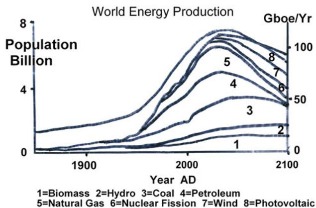
**Fig. 2** Estimates of world energy production projected into the future in a scenario [3]. Starting from the bottom, the shaded layers are respectively: Biomass, Hydro, Coal, Petroleum, Natural Gas, Nuclear Fission, Wind, and Photovoltaic. The topmost line is the projected world population
