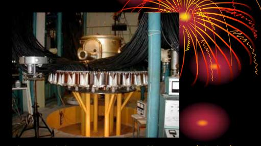
Capacitive storage (left) & chamber with current collector (right)  $W_{max} = 1.8 \text{ MJ}, V_{max} = 50 \text{ kV}, Mather-type}$
