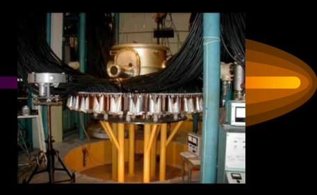
Capacitive storage (left) and discharge chamber with current collector (right)
