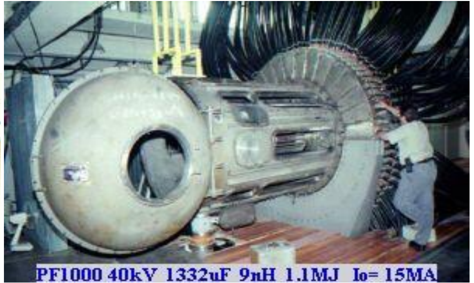
Figure 4b. 1 MJ PF1000 plasma focus
