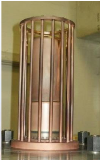
Anode = 10 cm OD Cathode = 15 cm ID Pyrex glass insulator
